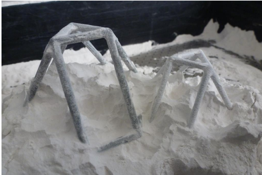
Figure 8: Models of different thickness for d = 19 being "excavated"
