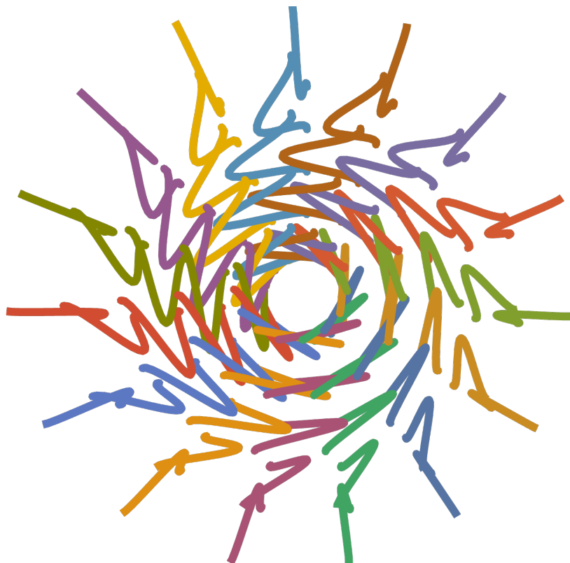
Figure 8.4: Torsionally buckled ASM - N_x = 0.5 , N_p = 0.1
