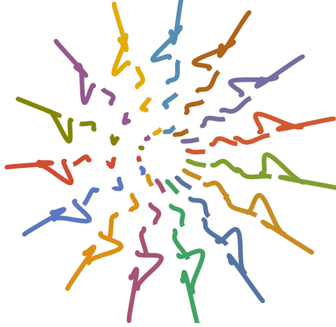
Figure 8.3: Torsionally buckled ASM - N_x = 0.4 , N_p = 0.1
